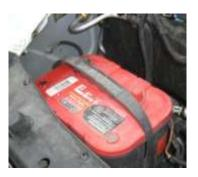
connected directly to the alternator and to the RV battery via the separator which connects the batteries together whenever the voltages present on ether battery indicates charging is taking place.
