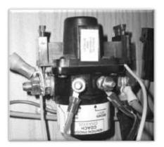
armature. When the coil is de-energized, the armature can move and the circuit is broken. Note that if you "push" and "hold" the rocker switch in the "off" position, the battery disconnect is closed while you hold the switch down.
